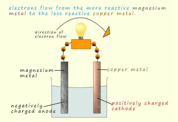
8. Explain why a simple cell using potassium and gold electrodes would produce a higher voltage than one using copper and zinc. Reference the reactivity series in your answer.
